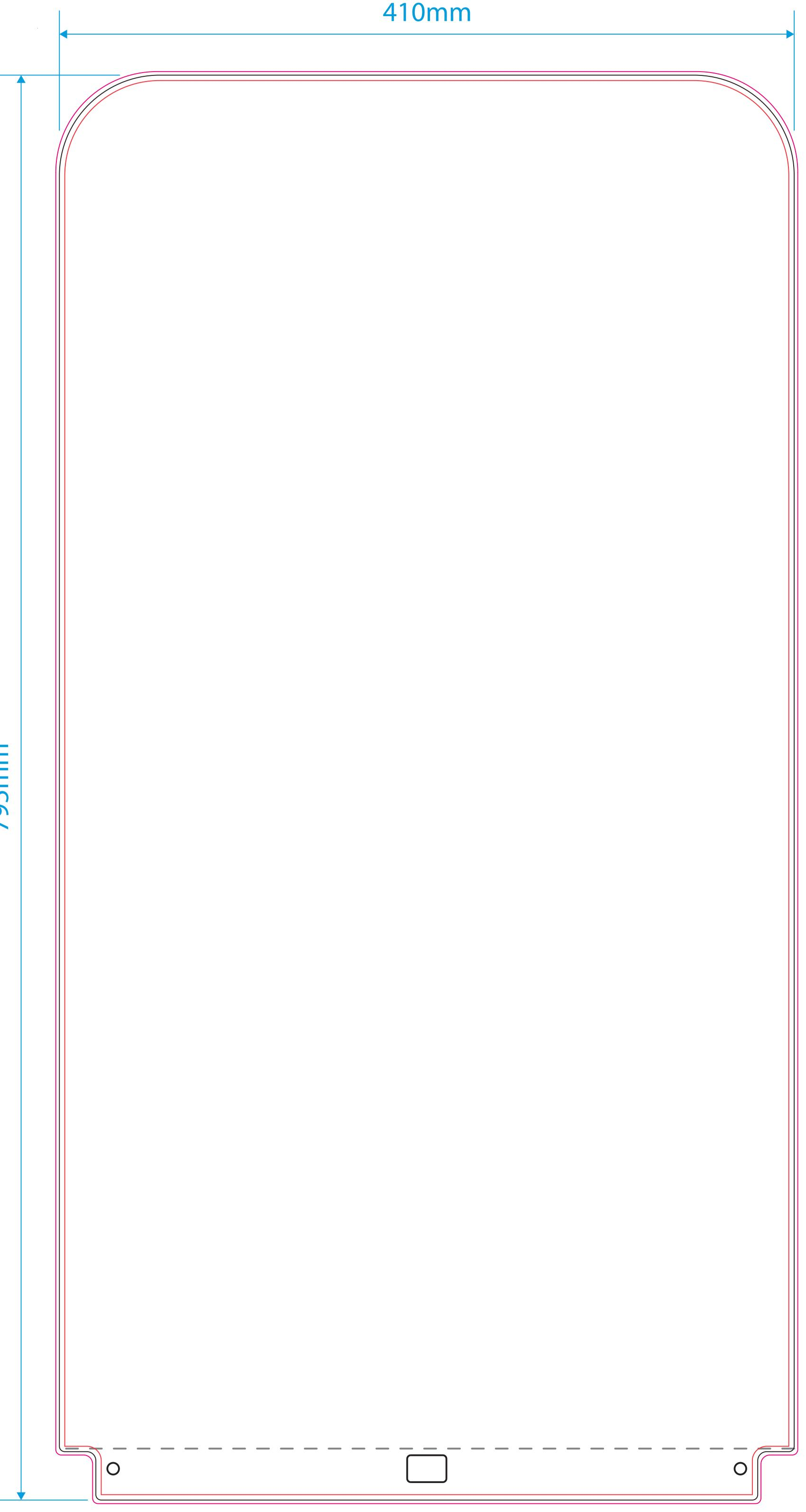
PLEASE NOTE: THIS AREA UNDERNEATH THE DASHED LINE IS NOT VISIBLE WHEN PANEL SLOTS INTO BASE.
